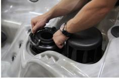
1. Turn filter housing ring counter-clockwise. Remove housing.
